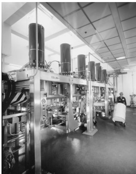
Fig. 6.17 Picture of an industrial SMB unit running at Aerojet in Sacramento (USA). Courtesy of Aerojet.
